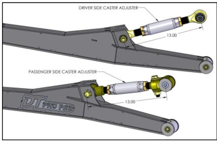
13. Remove the upper and lower control arms from the <u>driver side only</u> and save the axle mounting bolts, nuts and caster adjuster washer.
