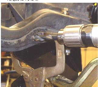
15. Drill pilot hole in cross-member to reattach brake line.
